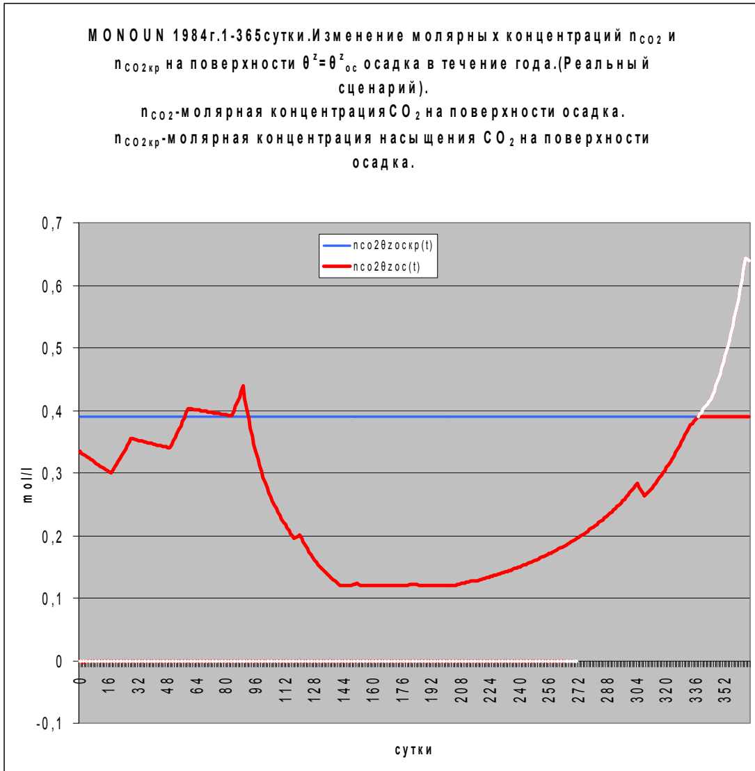
Fig. 11. MONOUN 1984.Day 1- Day 365. The Changing of the molar concentration n_{CO_2} and n_{CO_2кр} on the surfaces \theta^z = \theta^z_{oc} of the sediment stratum within one year.
